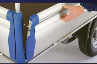
To release the Aluminium dropsides simply apply slight inward pressure to the dropside then lift the latch with fingers to release. The dropsides will only release when pressed inwards prior to the latch being lifted (Lifting the latch alone will not release the dropside).
