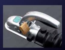
The lockable coupling head can be locked on or off the tow ball for additional security (Padlock not included).
