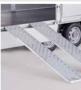
Perforated Steel Loading Skids 2.00m long with hook locking feature. Can be used on all trailer sides. A skid carrier may be purchased to store
