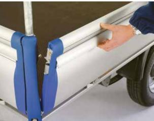
To release the Aluminium dropsides simply apply slight inward pressure to the dropside then lift the latch with fingers to release. The dropsides will only release when pressed inwards prior to the latch being lifted (Lifting the latch alone will not release the dropside).
